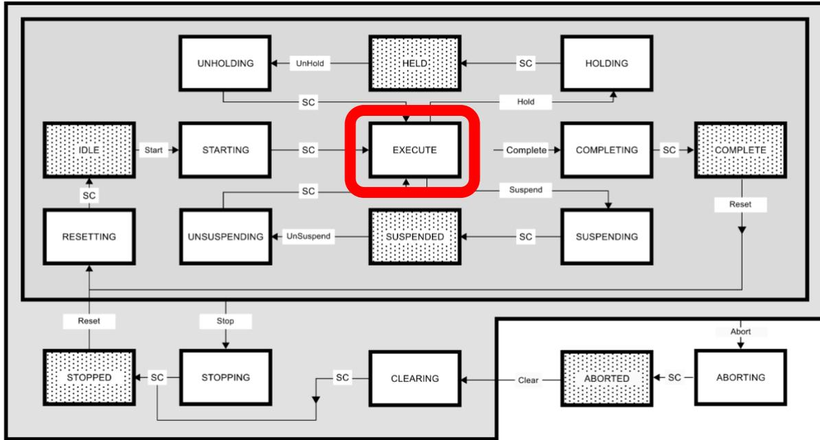
$$Performance = \frac{\text{Total Quantity Produced at this machine}}{\text{Time machine is producing Product(Execute) * Maximum Machine Speed}}$$
